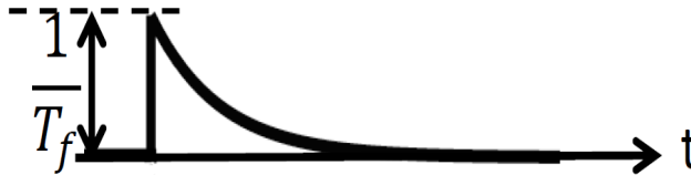
Figure 8.6 \delta -response of the RC integrator.
