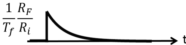
Figure 8.12 \delta -response of the active RC integrator. If we consider the voltage axis positive going up, this waveform should actually be flipped.
