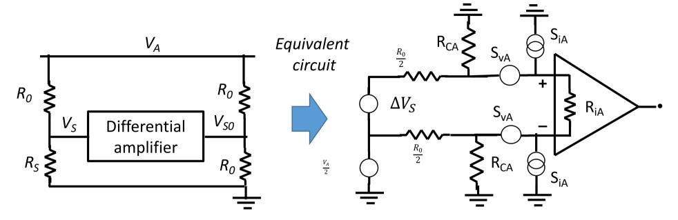
Since the **source resistance is low**, typically  $R_0$ =100  $\Omega$ :
