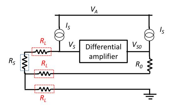
• Errors in  $\Delta V_S$  due to wire resistances  $R_L$  are avoided by a **«Three-wire-connection».** Both the reference arm and the RTD arm include in series a wire resistance  $R_L$ ; the third wire resistance  $R_L$  is inserted in the common return to the circuit ground
