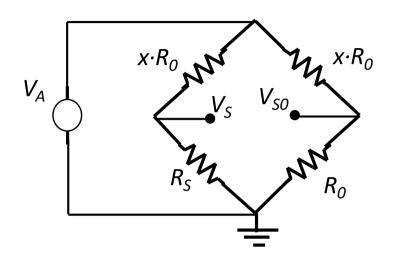
The Wheatstone bridge can be employed with **any ratio**  $\mathbf{x}$  of the voltage divider, i.e.  $R_S$  can be in series with a resistor  $\mathbf{x} \cdot R_O$  with any value of the factor  $\mathbf{x}$ . However, it is intuitive and readily verified that **with**  $\mathbf{x}=\mathbf{1}$  the highest output  $\Delta V_S$  is obtained
