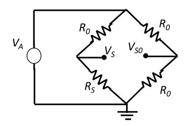
For small resistance variation  $\Delta R_S < 0.05 R_0$  the voltage variation  $\Delta V_S$  is approximately linear with  $\Delta R_S$  and can be computed by first-order development
