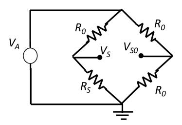
The cheap availability of integrated electronics for digital data processing and storage makes practical to extend the application of the Wheatstone bridge also to cases with **greater variations**  $\Delta R_S$ , that have a **non-linear but known dependance** of  $\Delta V_S$  on  $\Delta R_S$
