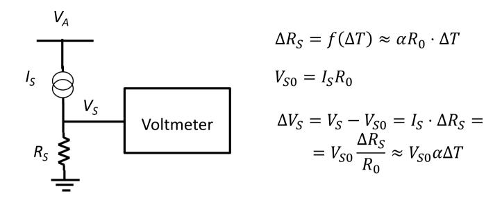
In modern electronics a simple approach is possible and practical thanks to the routine availability of current generators :
