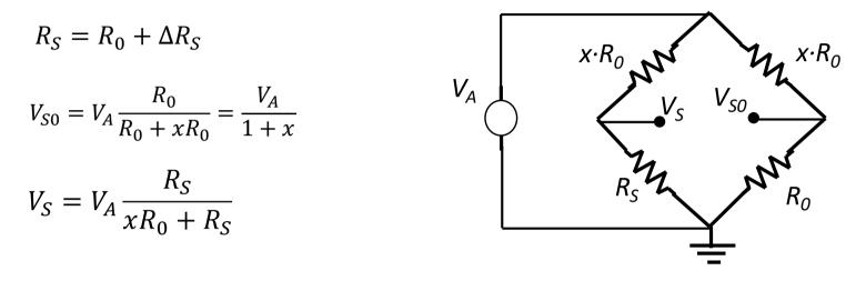
The Wheatstone bridge can be employed with **any ratio x** of the voltage divider, i.e.  $R_s$  can be in series with a resistor  $x \cdot R_o$  with any value of the factor **x**. However, it is intuitive and readily verified that **with x=1 the highest output**  $\Delta V_s$  is obtained
