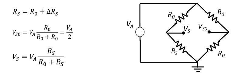
For small resistance variation  $\Delta R_s < 0.05 R_0$  the voltage variation  $\Delta V_s$  is approximately linear with  $\Delta R_s$  and can be computed by first-order development
