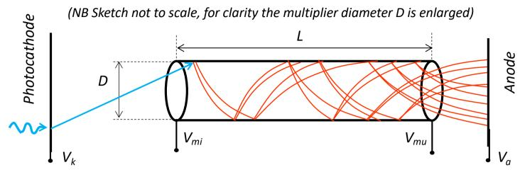
In order to get PMTs more simple, compact, robust and less sensitive to mechanical vibrations, minitubular electron multipliers were introduced (in the late years 60's)
