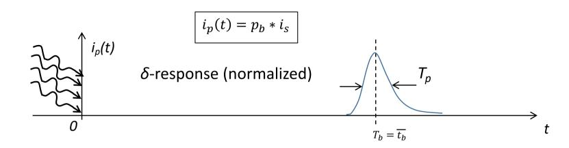
• The  $\delta$ -response is a convolution  $i_p = p_b^* i_s$ , hence its FWHM  $T_p$  is quadratic sum of FWHMs  $T_w$  and  $T_i$  of the components
