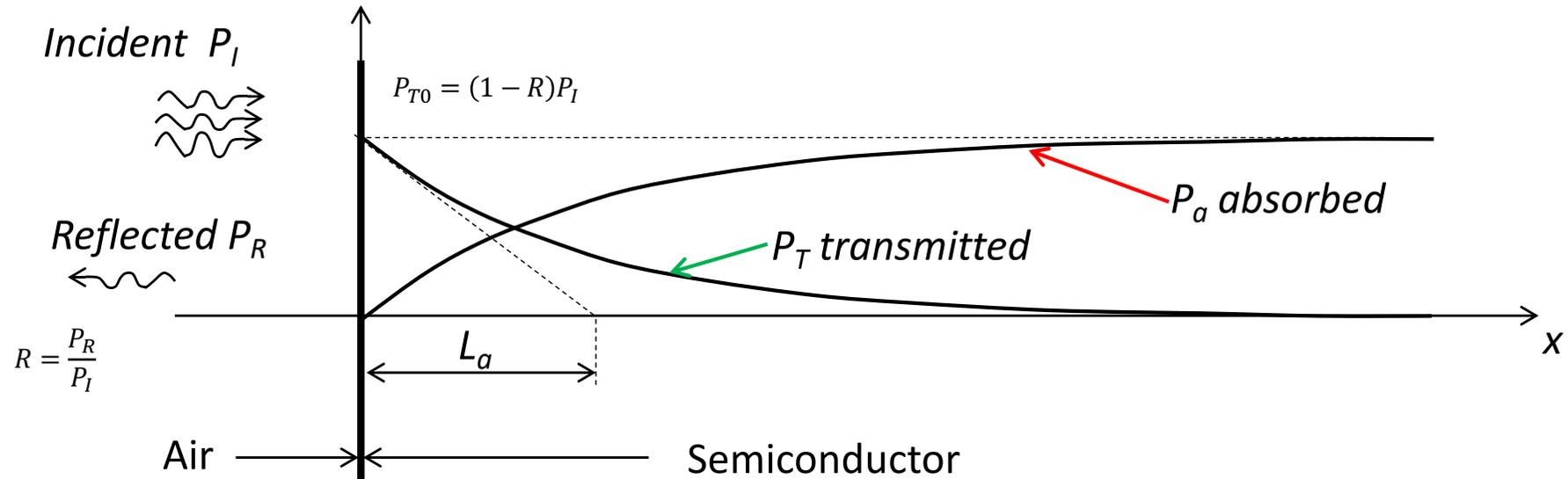
For moderate or low  $P_T$  the absorption in  $dx$  is proportional to  $P_T$  (linear optic effect)
