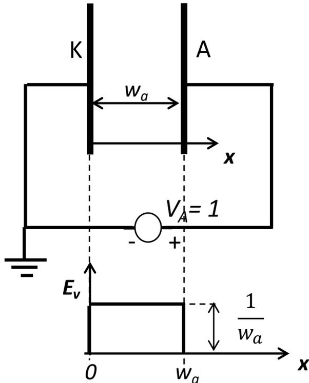
Reference electric  $E_v$  field computed with electron removed;  $V_A = 1$  ;  $V_K = 0$
