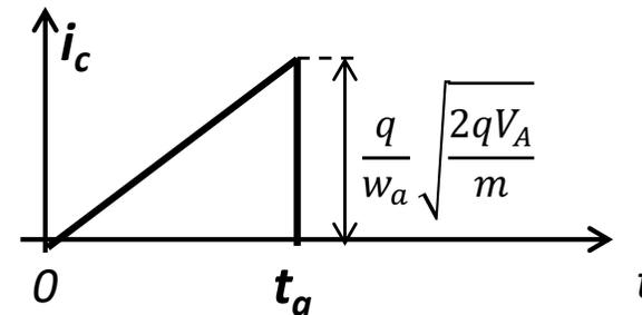
The frequency response is the Fourier transform of the SER pulse, which has a high frequency cutoff inversely proportional to the pulse width.
