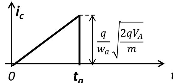
In a phototube with planar geometry the **single electron response (SER)** is a pulse with triangular waveform
