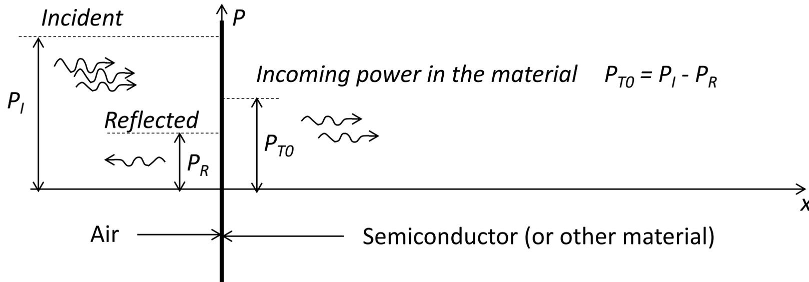
At the surface strong discontinuity of the refraction index  $n$ , from  $n = 1$  for air to  $n > 1$  for semiconductor: e.g. for silicon it is about  $n \approx 3,4$  and depends on the wavelength. This discontinuity gives a **high reflection coefficient  $R$**
