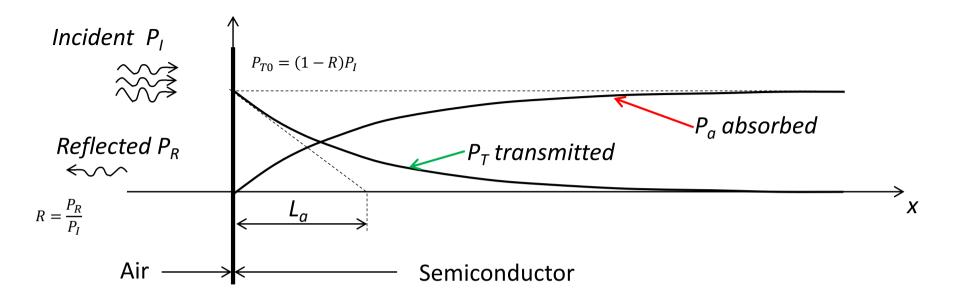
For moderate or low  $P_T$  the absorption in dx is proportional to  $P_T$  (linear optic effect)
