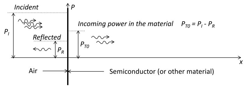
At the surface strong discontinuity of the refraction index n, from n = 1 for air to n > 1 for semiconductor: e.g. for silicon it is about  $n \approx 3,4$  and depends on the wavelength. This discontinuity gives a **high reflection coefficient** R
