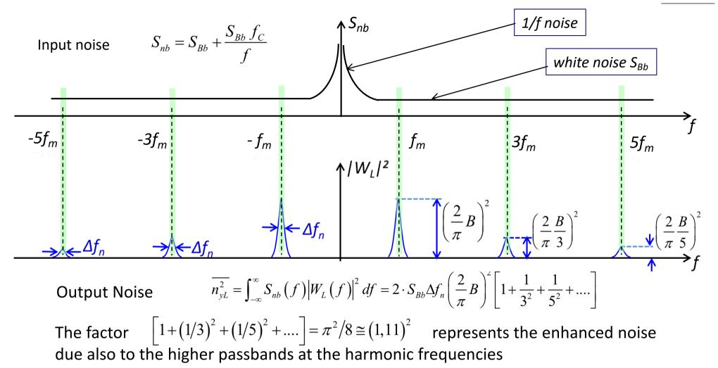
$$\overline{n_{yL}^2} = 2S_{Bb}\Delta f_n \left(\frac{2}{\pi}\right)^2 B^2 \frac{\pi^2}{8} = B^2 S_{Bb}\Delta f_n$$
