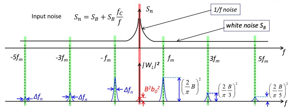
A squarewave with non-zero-mean generates a spurious band at f=0 with additional noise
