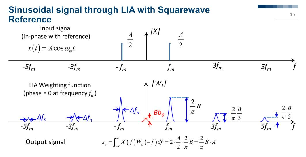
NB This is easily verified in time, since: LIA output y(t) = time average of  $z(t)=x(t)\cdot B m(t)$  = mean of the in-phase component of the sinusoidal input rectified and multiplied by B
