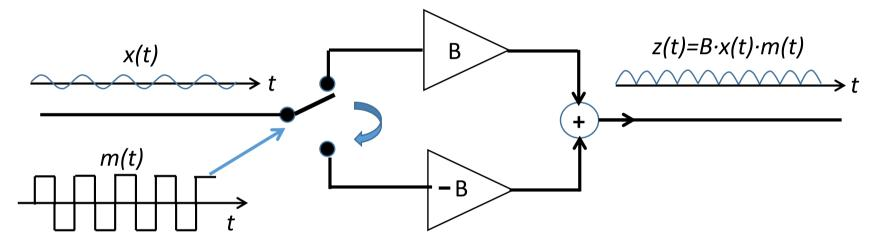
The noise referred to the input, the linearity and the dynamic range of these circuits are remarkably **better than those of analog multiplier circuits** (even high-performance types) because they are limited just by the performance of amplifiers and switch-devices.
