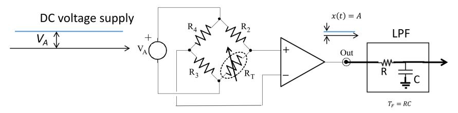
Let us consider the set-up of the key example (measurement with resistive sensor) now with DC supply voltage  $V_A$  equal to the amplitude of the previous AC supply. The signal now is a DC voltage equal to the amplitude A of the previous AC signal.
