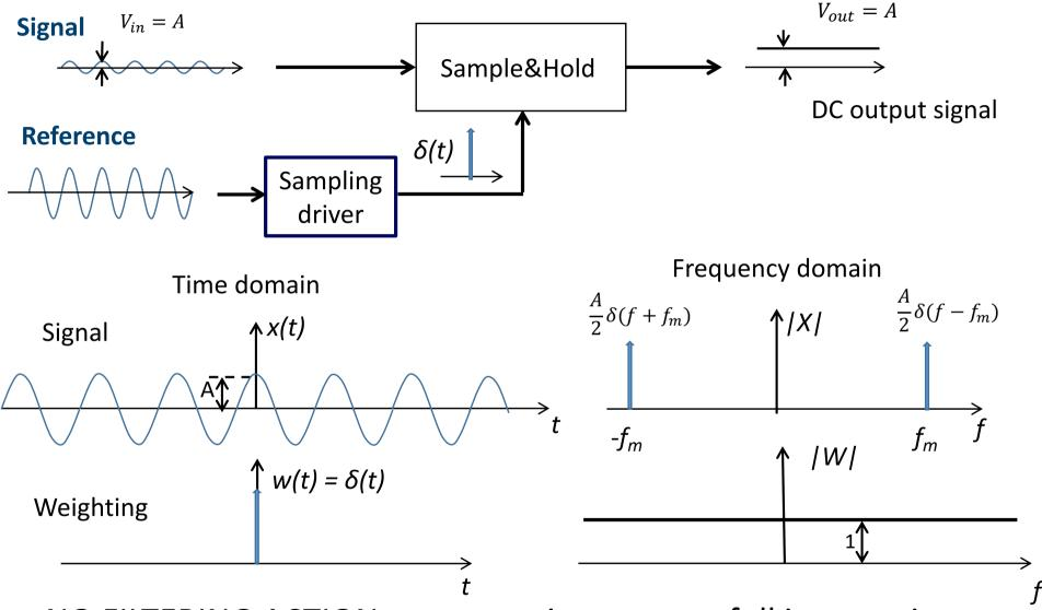
NO FILTERING ACTION: output noise power = full input noise power
