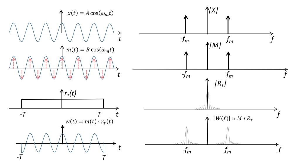
TRULY EFFICIENT FILTERING : just one narrow band at  $f_m$
