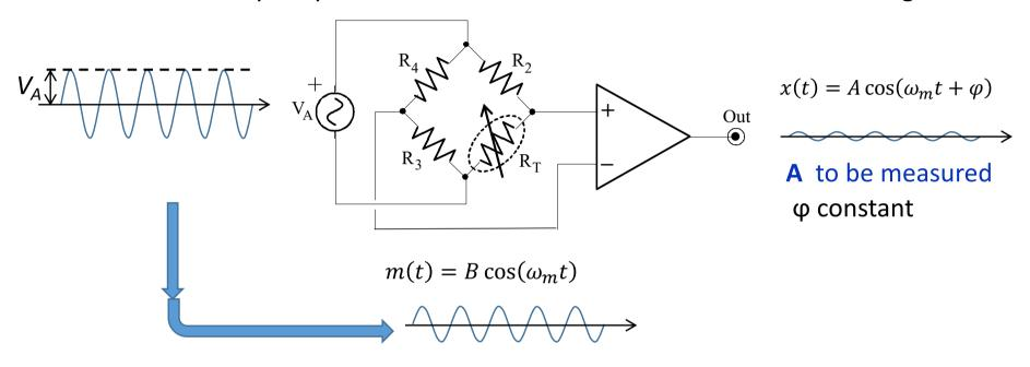
$R_T$  e.g. strain sensor, the resistance varies following a mechanical strain  $\boldsymbol{\vartheta}$
