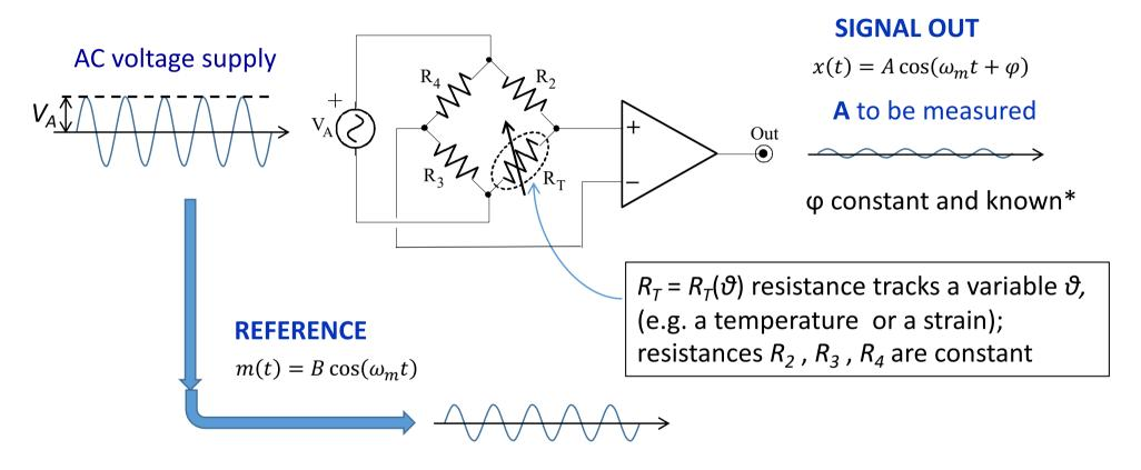
Shows the frequency and phase of the signal i.e. points out the peak instants of the signal
