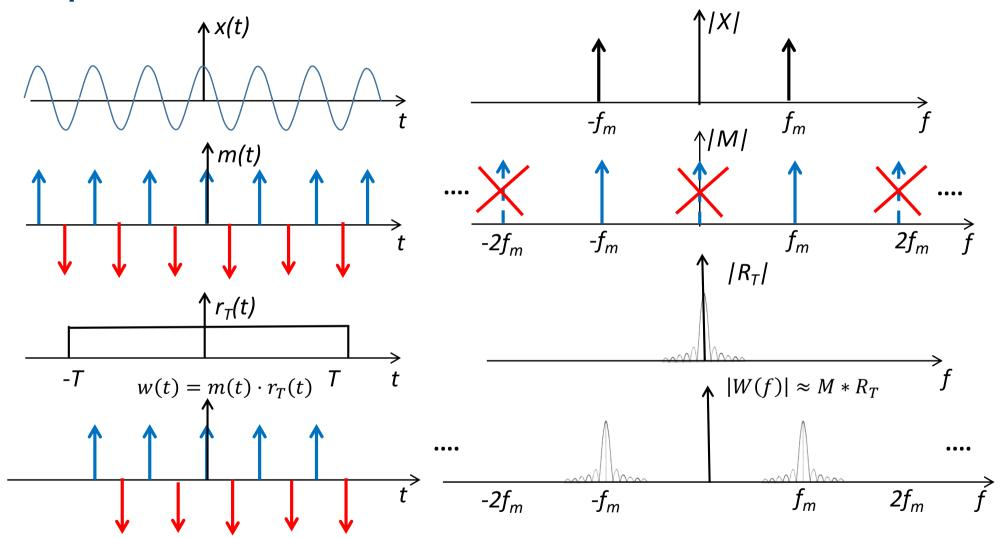
FILTERING: narrow bands at  $f_m$  and at **odd** multiples  $3f_m$ ,  $5f_m$  ....
