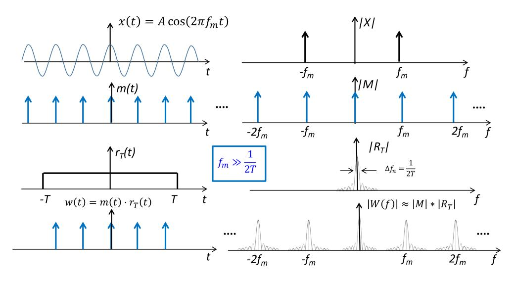
FILTERING: narrow bands at frequencies 0,  $f_m$ ,  $2f_m$ ,  $3f_m$ ....
