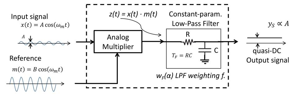
The **constant** parameter LPF performs a **running** average of the output z(t) of the demodulator. The output is continously updated and tracks the slowly varying amplitude A(t). This basic set-up is denoted Phase-Sensitive Detector (PSD) and is the core of the instrument currently called **Lock-in Amplifier**.
