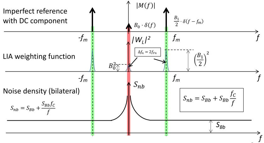
The ratio  $\widehat{S_{nu}}/S_{Bu} > f_C/f_{Fn} \gg 1$  can match or exceed the amplitude ratio  $\frac{B_1^2}{2B_0^2}$  so that the noise in the fake passband  $\overline{n_{yL0}^2} = B_0^2 \cdot \widehat{S_{nb}} \cdot \Delta f_n = B_0^2 \cdot \widehat{S_{nu}} \cdot f_{Fn}$  can equal or exceed that in the correct passband  $\overline{n_{yL1}^2} = \frac{B_1^2}{2} \cdot S_{Bb} \cdot \Delta f_n = \frac{B_1^2}{2} \cdot S_{Bu} \cdot f_{Fn}$
