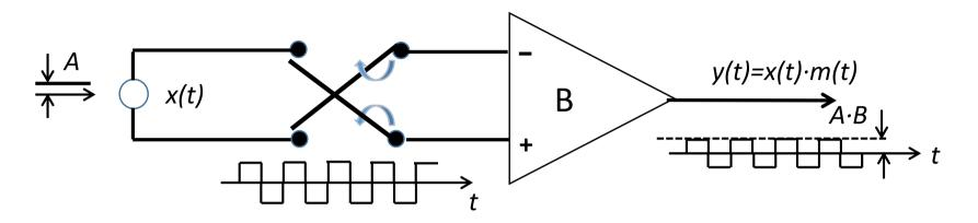
Switching example: chopper (ON-OFF modulation)
