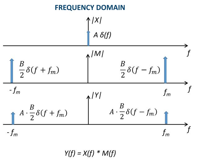
The signal is shifted in frequency by  $+f_m$  and  $-f_m$ and in phase by  $+\varphi_m$  and  $-\varphi_m$  respectively 20
