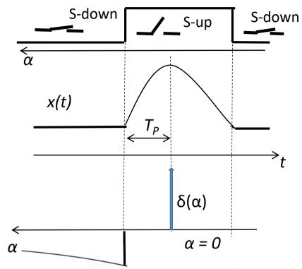
BLR principle is alike filtered zero-setting, but with a basic advantage: much shorter  $T_P$  much higher band-limit  $f_{if}$  (high-pass)
