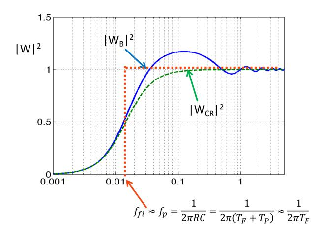
LIN –LOG DIAGRAM highlights 1/f noise power  $\propto$  area of  $|W|^2$
