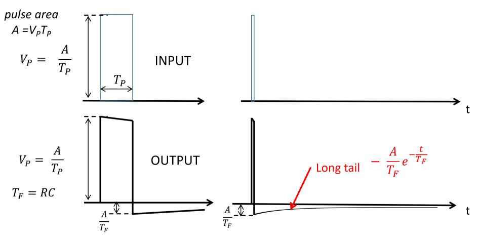
NB: DC transfer of CR is zero → net area of the output signal is zero
