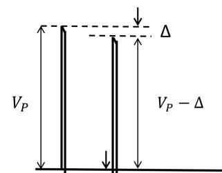
A pulse that follows a previous one within a fairly short time interval ( $T_D < 5 T_F$ ) steps on the slow tail of the first pulse. Therefore, it **starts from a down-shifted baseline**, so that the amplitude measured for it is smaller than the true one.
