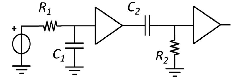
$$|W|^2 = \frac{1}{1 + (2\pi f R_1 C_1)^2} \cdot \frac{(2\pi f R_2 C_2)^2}{1 + (2\pi f R_2 C_2)^2}$$
