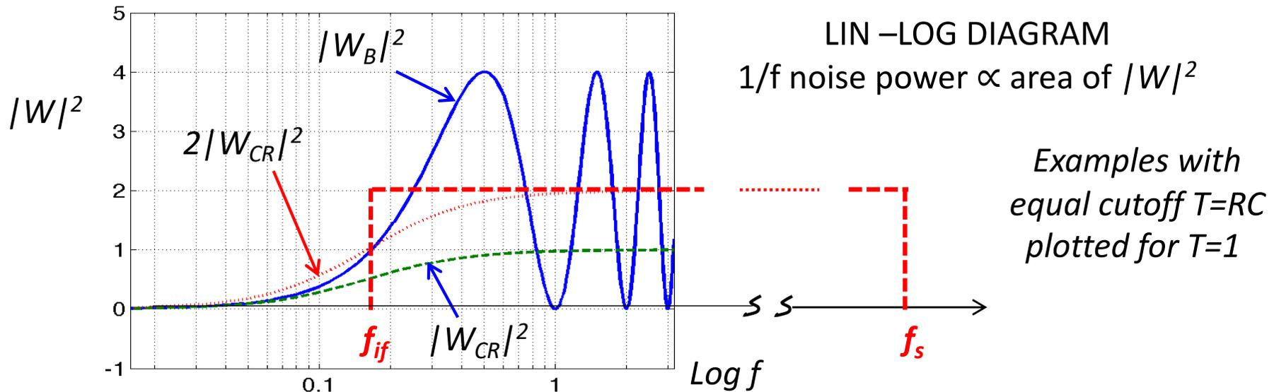
1/f noise power  $\overline{n_f^2}$  limited also by a low-pass  $f_s$ , but with  $f_s \gg 1/T$  ( $f_s \gg 1/RC$ )
