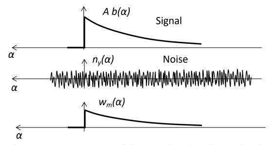
The best result in measurements of the amplitude of signal pulses accompanied by **stationary** white noise is obtained with weighting function equal to the signal shape. This conclusion is intuitive: since the noise is uncorrelated, the output noise power is the weighted sum of the noise instantaneous power at all times; since this power is equal at all times, it is convenient to give higher weight when the signal is higher.
