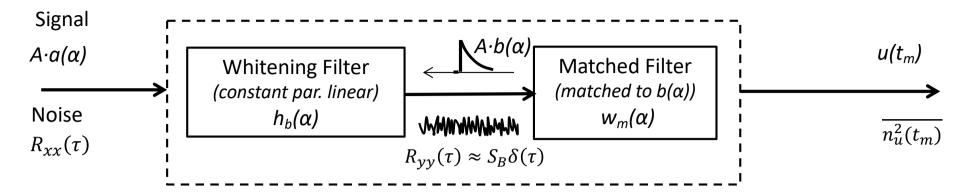
• for a given stationary noise, it is always possible to find a **constant-parameter** linear filter that produces such a result, since it has transfer function  $H_b(f)$  such that
