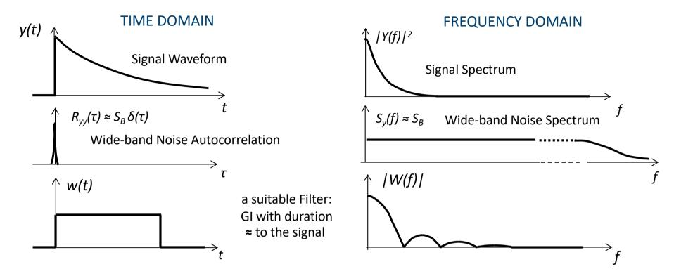
For a measurement of pulse amplitude, a filter has to collect most of the signal and reject most of the noise. It's intuitive that its action should be:
