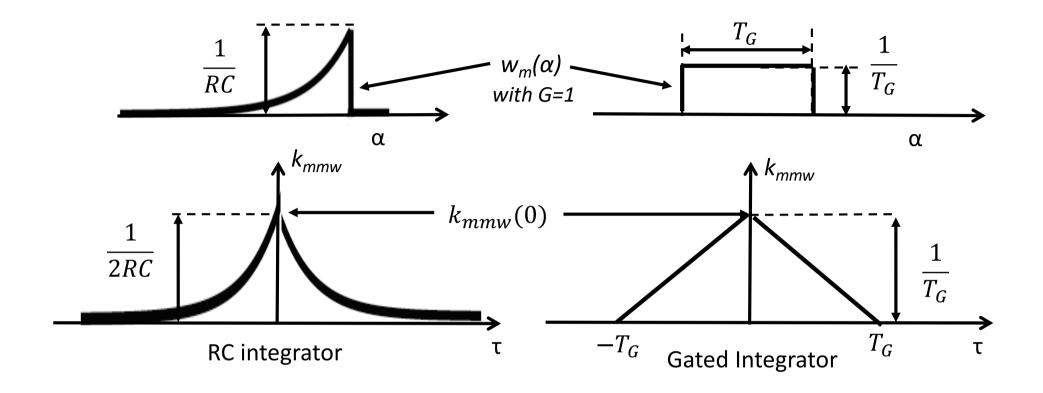
We consider here filters with equal DC gain of unity, hence with equal output signal.
