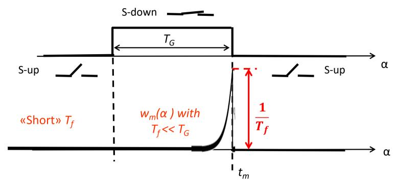
The S&H has unity DC gain (C is fully charged at the input voltage within  $T_G$ )
