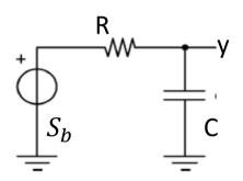
this is just the noise generated and self-filtered by a constant parameter RC filter and is INDEPENDENT OF THE R VALUE, in agreement wth the S&H circuit model.
