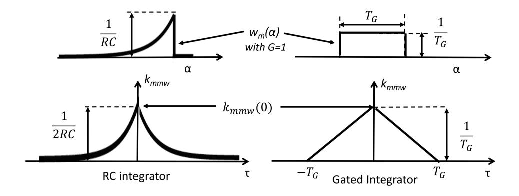
We consider here filters with equal DC gain of unity, hence with equal output signal.
