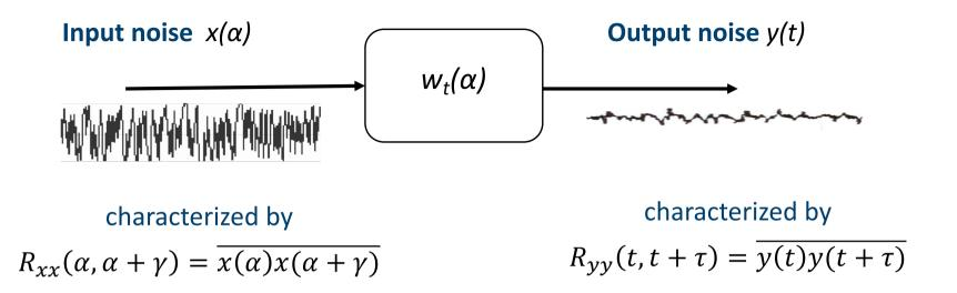
The **output autocorrelation** can be obtained in terms of the **input autocorrelation** and of the filter **weighting** function :
