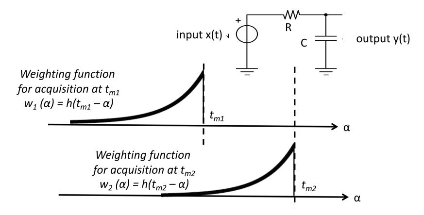
For constant-parameter filters the weighting function for any  $t_m$  has
