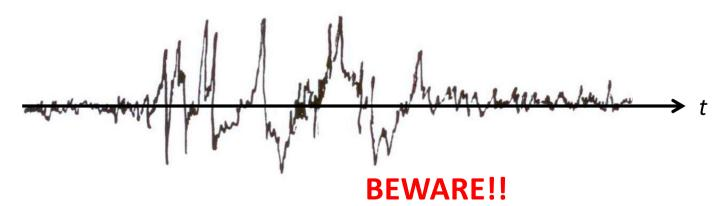
the probability density **p** alone does not give a complete description of the noise, in fact <u>different cases</u> can have <u>equal probability</u> density **p**
