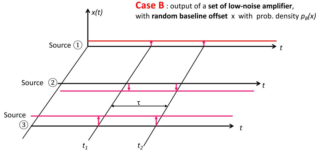
Values  $x(t_1)$  and  $x(t_2)$  measured on a sample waveform at different  $t_1$  and  $t_2$ :
