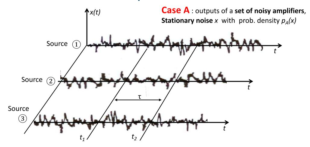
Values  $x(t_1)$  and  $x(t_2)$  measured on a sample waveform at different  $t_1$  and  $t_2$  are random values with equal probability density  $p_A(x)$  and they are:
