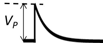
Exponential pulse:  $x(t) = V_P e^{-t/T_P}$        $X(f) = V_P T_P \frac{1}{1+j2\pi f T_P}$
